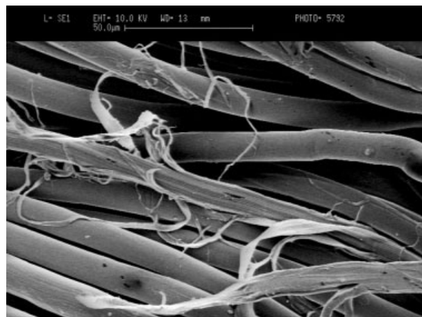
Figure 8 Mild fibrillation observed in Reaktant DH treated sample after five washes.
