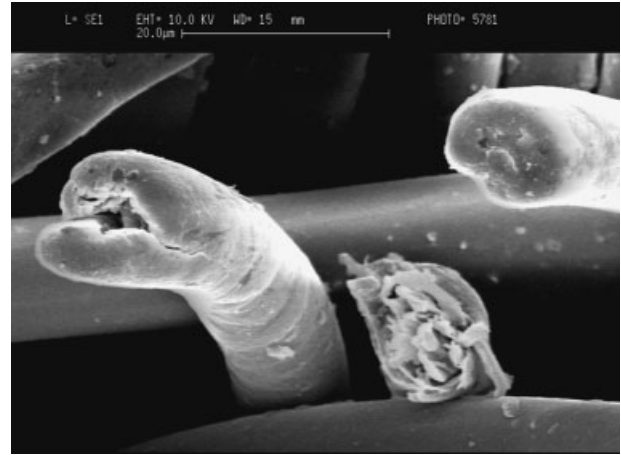
Figure 2 Multiple splitted, rounded, and axially split rounded fiber ends (untreated Tencel fabric).
